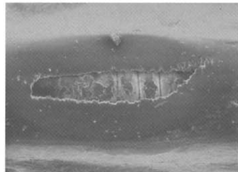
Fig. 12 Creep failure of a silicone rubber lead
