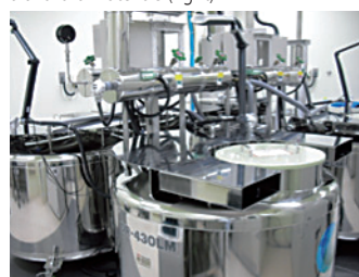
Automatically supplied liquid nitrogen cell storage tank
