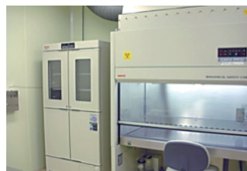
A cold box for medicinal use with a freezer (left) and a safety cabinet that can accommodate biohazard materials (right)
