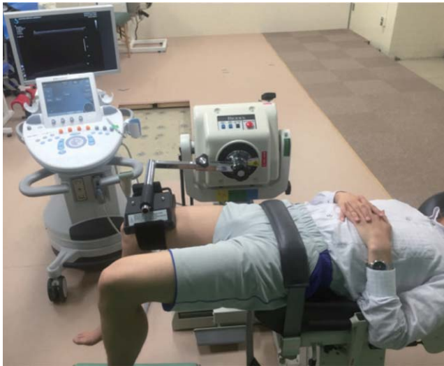
Fig. 3. The subject was in a supine position on the seat of BIODEX. The pelvis was fixed to the BIODEX using a strap. The pad of BIODEX was attached to the distal position of the thigh on measurement side. The angle of the knee on the measurement side was varied in accordance with gravity. The hip flexion angle of the contralateral side was 0° and knee flexion angle was 90°.
