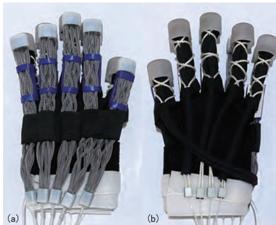
Figure 1. The developed wearable robot. Dorsal (a), palmar (b).
