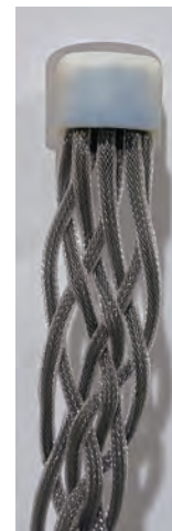
Figure 3. Flat-braided design. Seven interwoven artificial muscles for extension are attached to the back of the hand.
