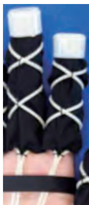
Figure 2. Three-point bending structure. The intersections of the artificial muscles for flexion that are wrapped around the fingers are located on the distal interphalangeal (DIP) joint, proximal interphalangeal (PIP) joint, and metacarpophalangeal joint.
