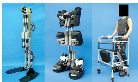
Figure 2. WPAL (Wearable Power-Assist Locomotor). The robots for gait reconstruction of patients with paraplegia. WPAL has 6 motors for each hip joint, knee joint, and foot joint mounted on a medial system-like frame. The special walker equipped with a motor control circuit and battery guarantees patient safety and reduces the burden on the patient. Patients can operate the WPAL using 2 lever switches and 2 button switches on the walker, and can wear and remove the WPAL by themselves after some training.
